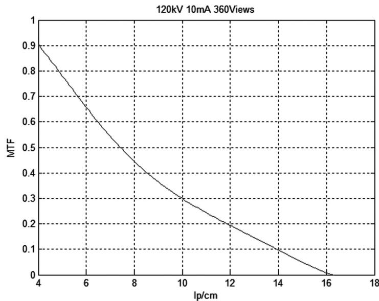
Fig. 3. MTF Curve of the optimal protocol (120 kV/10 mA and PVno.360).10% MTF was 13.9 lp/(359.7  $\mu$ m).
